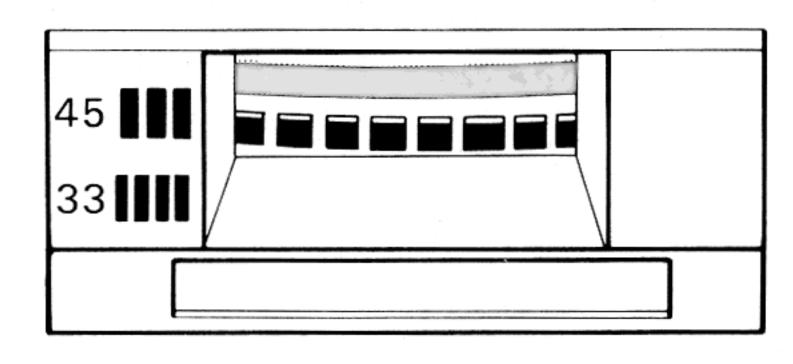
● The neon lamp is energized by a 120 Hz pulse from the builtin crystal oscillator and assures precise speed indication regardless of any line-frequency deviation.
