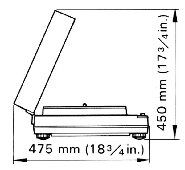
The turntable has resilient feet that isolate the mechanism from external shock and vibration. Use them in locked position, but when placing the turntable on an uneven surface, turn eachfoot until the unit is level.
