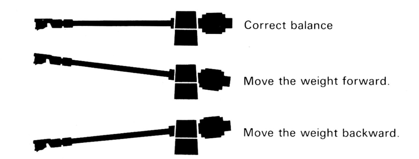
While holding the Counterweight at the balanced position, separately turn the Tracking-force Ring until the "0" indication meets the center line on the Tonearm. Recheck the balance.
