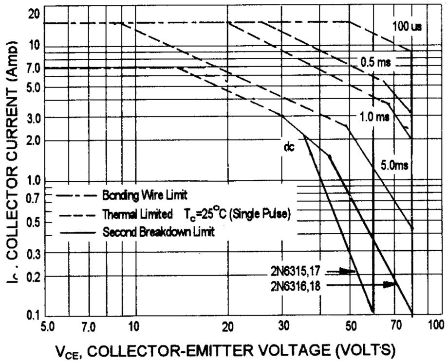
There are two limitation on the power handling ability of a transistor: average junction temperature and second breakdown safe operating area curves indicate  $I_C$ - $V_{CE}$  limits of the transistor that must be observed for reliable operation i.e., the transistor must not be subjected to greater dissipation than curves indicate.
